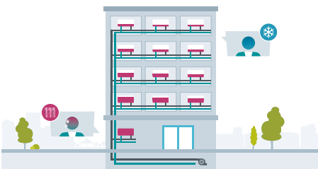
Static hydronic balancing: Uneven energy distribution under part load conditions.
